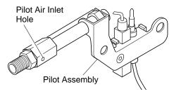
Figure 23 - Pilot Inlet Air Hole
